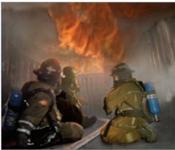
Thermal layering, as observed in the chamber.
